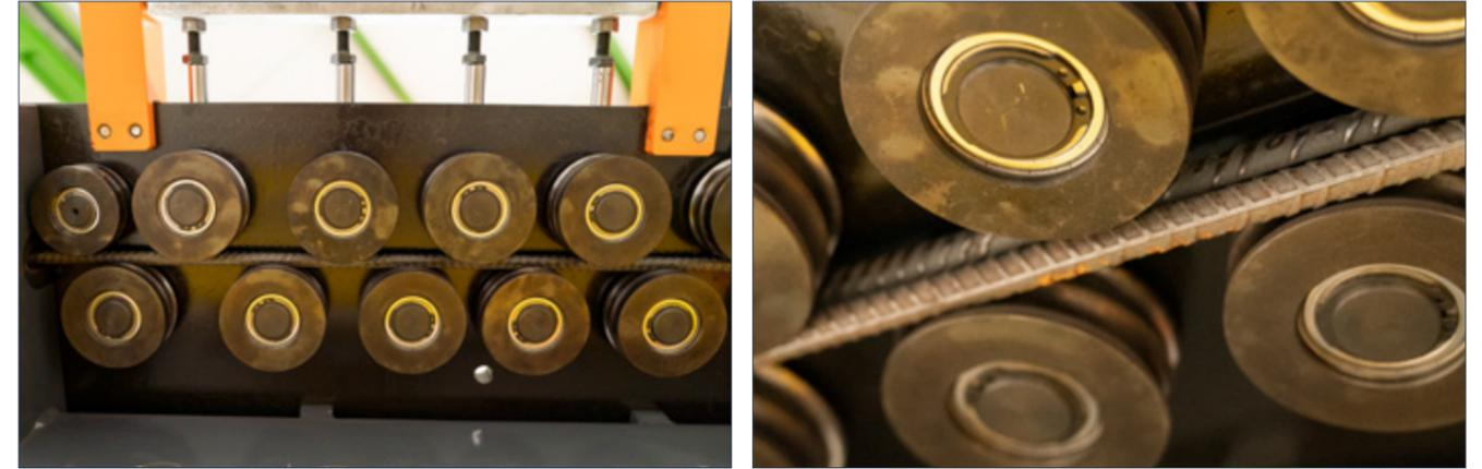
Straightening wheels are produced by most quality material with heat treated. It makes the machine firstly then parts very agile.
